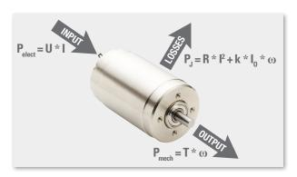
The efficiency is defined by the ratio of the mechanical power and the electrical power:  $\eta = P_{\rm mech} / P_{\rm elect}$
