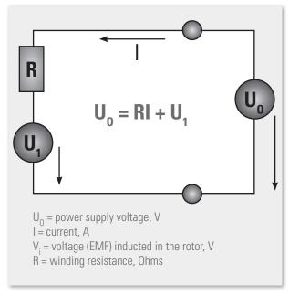
The voltage induced in the rotor is proportional to the angular velocity of the rotor:
