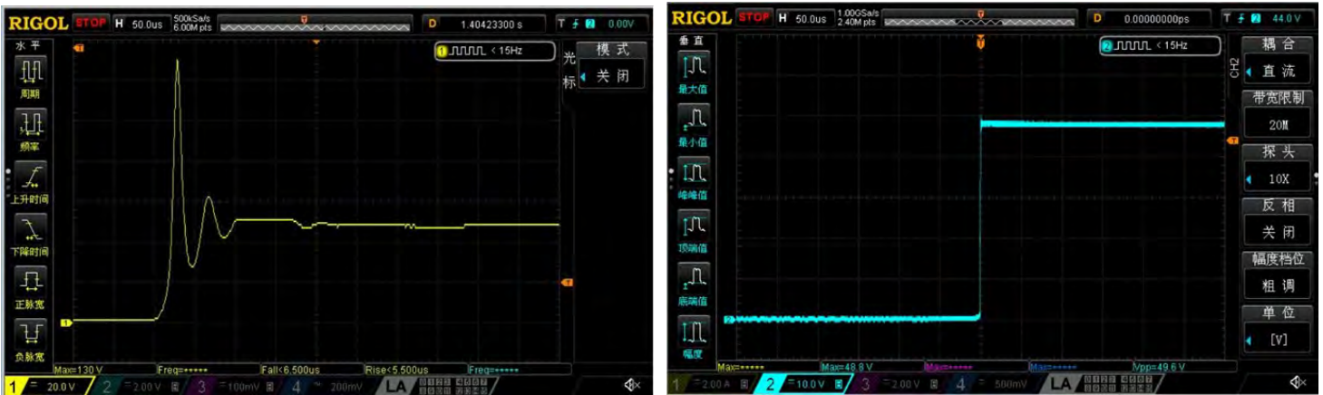
(a) Abnormal Power Input Voltage Waveform ( V_{max} = 130V > 60V )
