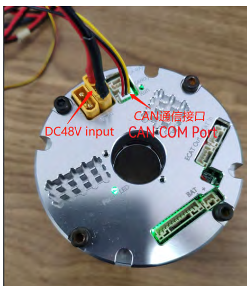
(a) CAN wiring
